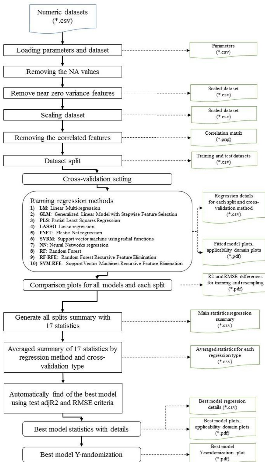
Figure 18 RRegrs methodology flowchart. The main steps followed by the RRegrs function are indicated as well as the input parameters needed and the format of the output produced
