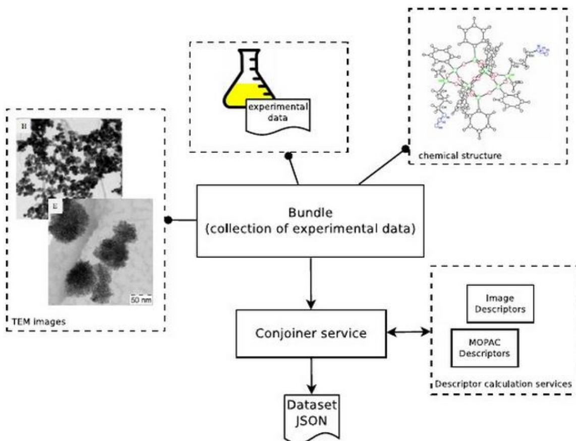
Figure 2 Conjoiner API: modelling-oriented information can be extracted from bundles of experimental data.
