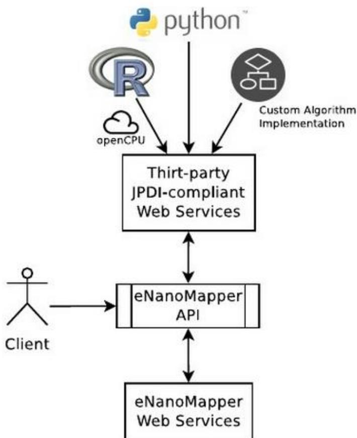
Figure 7 JPDI-compliant web services can be seamlessly incorporated into the eNanoMapper framework.
